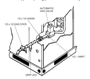
FIGURE 5 - EXTERNAL SUPPLY CONNECTION EXTERNAL SHUT-OFF
